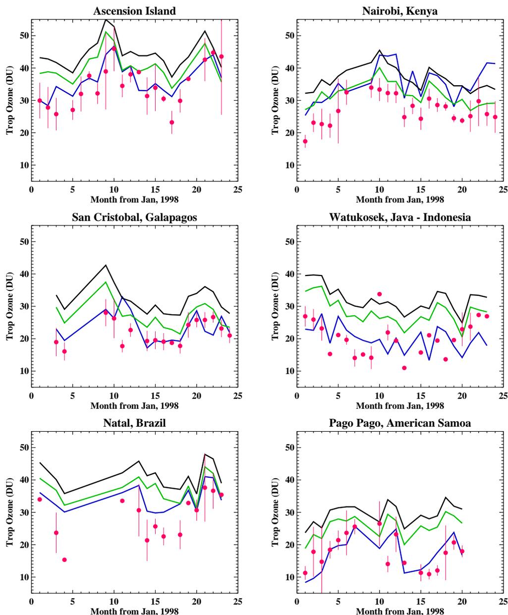
**Fig. 6.** Comparison of CCD and CCP tropospheric ozone with SHADOZ tropospheric ozone from 1998–2000 at six sites. Red circles are the sonde integrated tropospheric ozone columns, vertical bars represent 1 SD of the ozonesonde monthly mean, black lines represent the CCD tropospheric columns, blue lines represent the derived CCP tropospheric columns, and green lines are the CCD results after applying the correction from the cloud anomalies offset between Nimbus-7 / EP TOMS.
