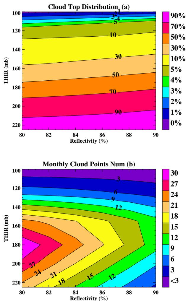
**Fig. 3.** (a) The THIR cloud-top distribution as a function of reflectivity for pressures less than 225 hPa, and (b) the monthly average number of cloud points between 1979–1984 as functions of THIR pressure and reflectivity.
